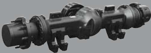
Highly durable split type drive axle
